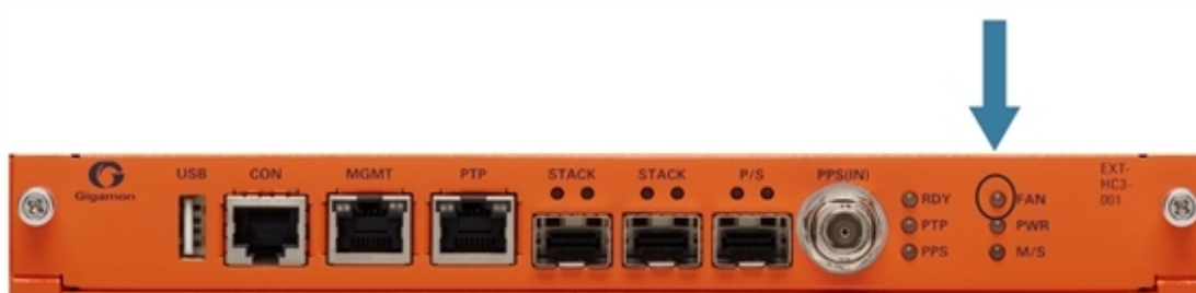
Figure 5 Global Fan LED Location on GigaVUE-HC3 Front
