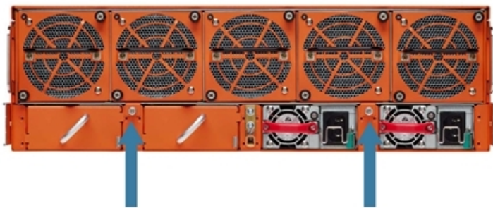
Figure 10 Fan Tray Screw Location on GigaVUE-HC3 Rear
